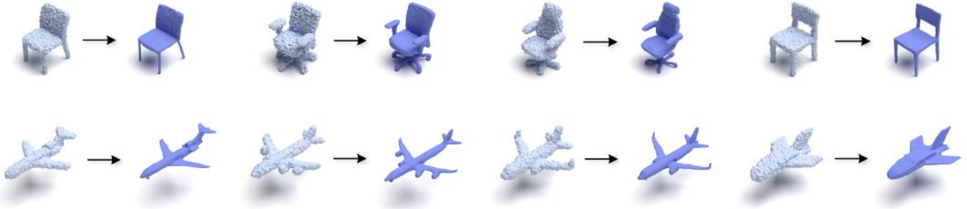
Fig. 12. The results of reconstructing surfaces from the point clouds generated on the Chair and Airplane categories.
