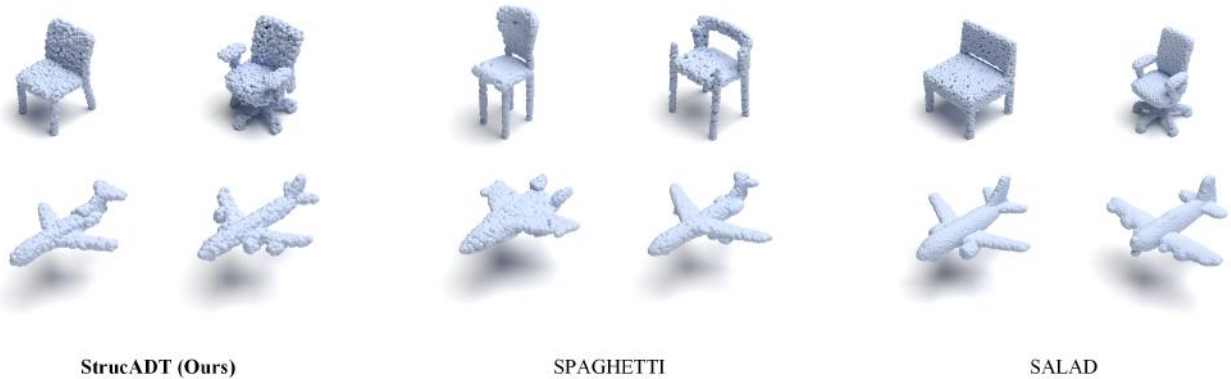
Fig. 7. Comparison results of generated 3D point cloud shapes between our method (StrucADT) with pre-trained 3D shape generation methods: SPAGHETTI and SALAD on the Chair and Airplane categories of the ShapeNet dataset.
