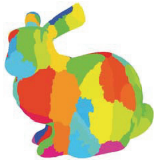
Fig.4. Bunny model with 69674 faces, which is partitioned to 100 segments.
